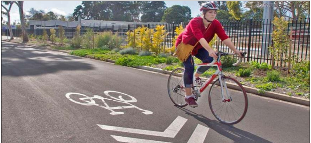
Figure 16 Typical sharrow treatment (source: dpti.sa.gov.au )
